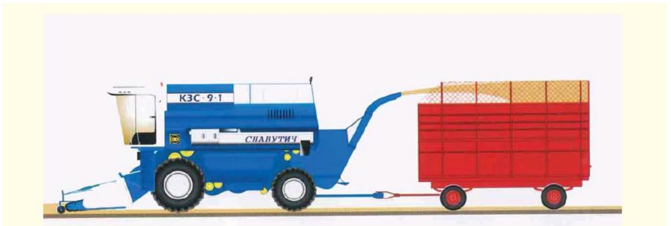
Fig. 4. Collecting straw by the “ streaming ” technology [16]
