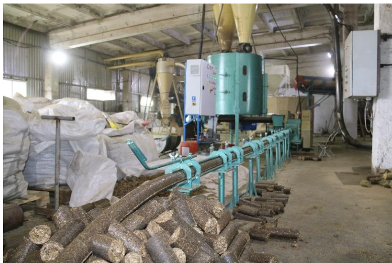
Fig. 4.5. Straw briquetting line with press Wektor BT-60.
