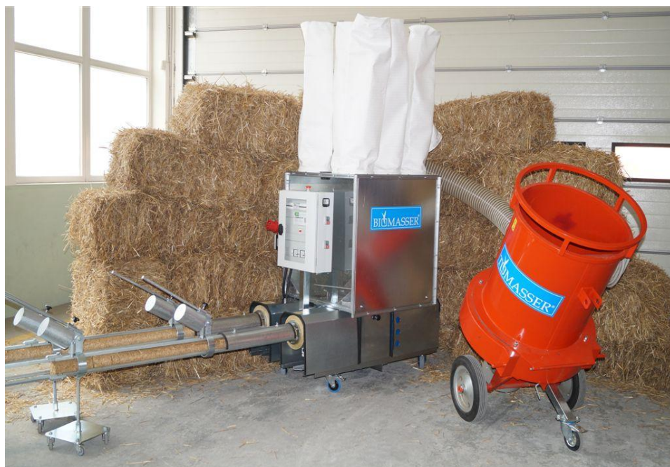
Fig. 4.3. Briquetter BIOMASSER DUO with comminutor TOMASSER RK.
