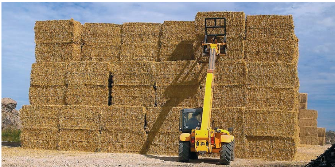
When using a telescope loader the bales can be stacked significantly higher than with a fork lift truck and a front loader.
