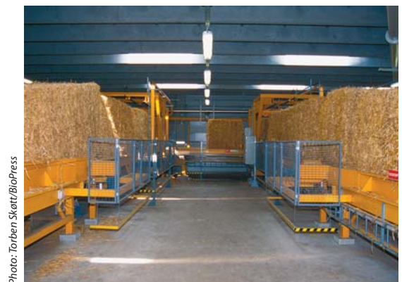
The bales of straw are transported to the shredders via conveyor belts – also called straw lanes.
