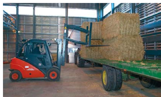
Unloading of straw at Thisted district heating plant. Notice that the forklift truck is capable of collecting the bales of straw, which are furthest away. When using a regular forklift truck the unloading must take place from both sides of the vehicle.
