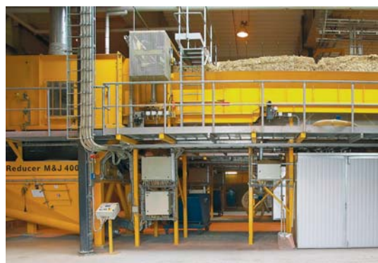
Big bales are taken to the straw cutter at Køge Bio Pellet Factory.
